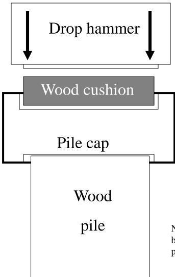
The cushion-pile cap combination serves as a "shock absorber", blunting the sharp force loading on the pile at impact.
