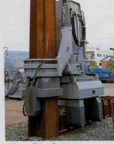
Silent Piler for H-section Steel Piles Only
