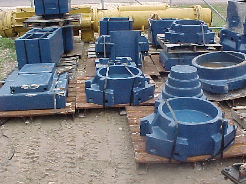
Drive Cap Layout (diesel hammer)
