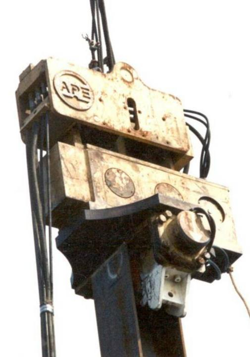
Driving **H-Beams** with a vibro fitted with a 90 degree turning plate
