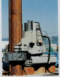
Silent Piler for Steel Tubular Piles Only
