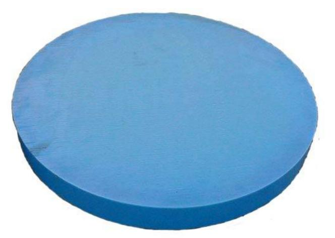
Nylon cushion material 2 inch thick in various diameters Use on D30 and smaller type hammers Switch to aluminum and conbest on larger hammers
