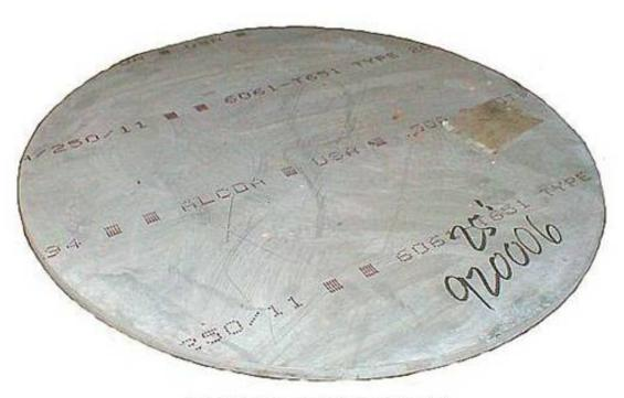
Aluminum cushion material 1/2 thick plates in various diameters
