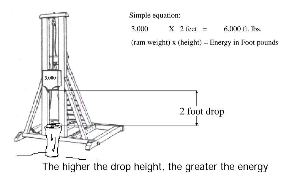
A drop hammer weighing 3,000 lb. falling from 20-feet with no bounce at impact would deliver 60,000 ft-lbs of energy.
